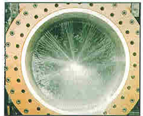
The water jets strike each other, not the interior of the sleeve.
