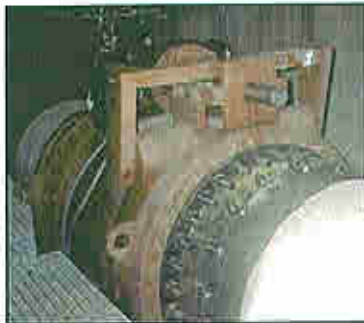
Model 711 Axial Flow Sleeve Valve with 36 inch flanges and sleeve
